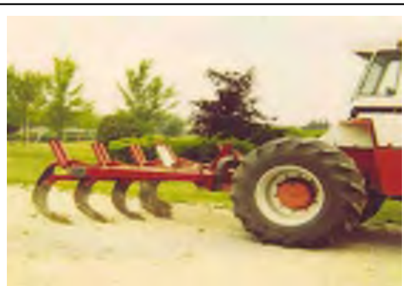
Fig. 7. One of several variations of an agricultural ripper. This unit has long, rugged shanks mounted on a steel V-frame for deep, aggressive fracturing through Phase 1.
